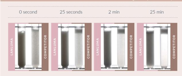
Both products were manually mixed for 1 minute before resting at room temperature.
